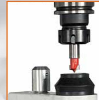
Quick set-up and no error thanks to the tool length pre-setting unit
