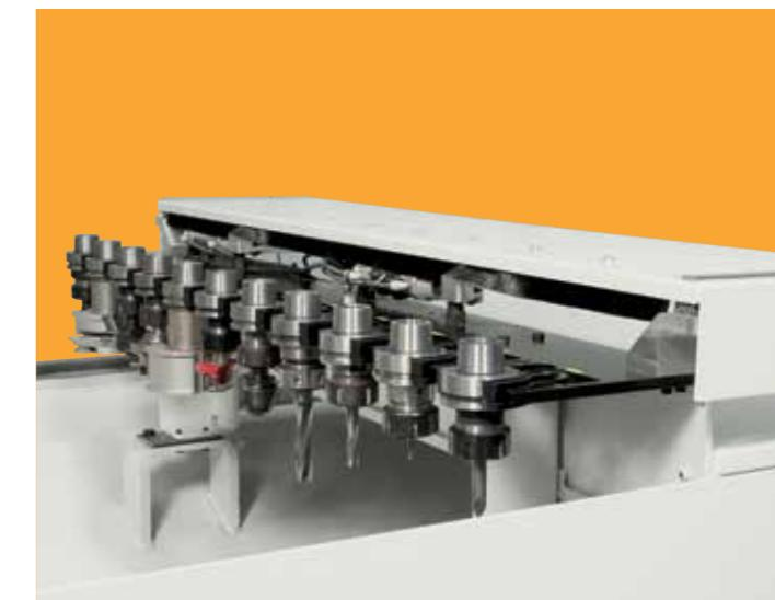
BT 16: quick and precise, the tool changer is placed on the Y carriage and allows a rapid tool change during the processing phase.
